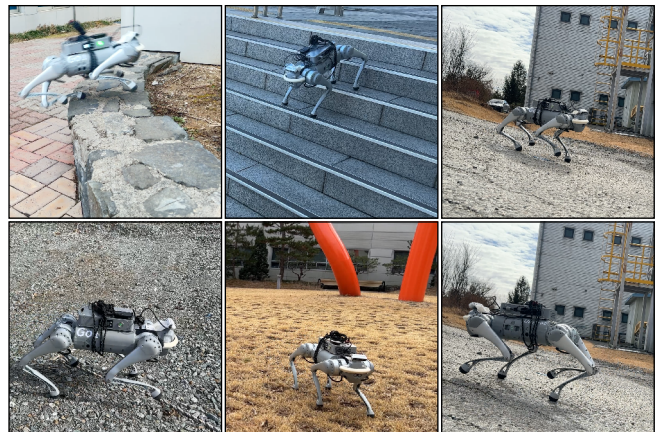
Fig. 6: Outdoor deployment snapshots: curb climbing on stone terrain, stair descending, slope descending, gravel walking, grass walking, and slope ascending.
